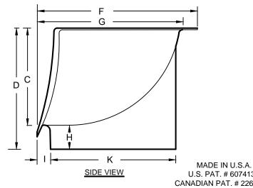
THE "24/12" BOWL WILL SERVICE UP THROUGH FULL 16" INLETS. THE "24/15" BOWL WILL SERVICE UP THROUGH FULL 18" INLETS. CAN BE USED FOR 21" MODERATE FLOW INLETS. ALL SIZES ARE FOR RETROFIT OR NEW CONSTRUCTION. FABRICATED IN MARINE GRADE FIBERGLASS AND FINISHED IN BRIGHT WHITE GEL COAT.
